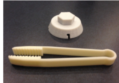
The plastic tools above were printed with the Made In Space 3D printer and are representative of tools used by the space station crew.
