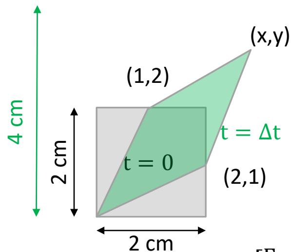
Find out the deformation gradient for the given deformation illustrated in the left figure.
