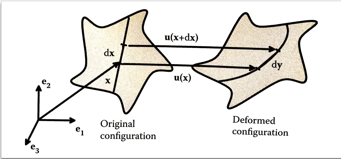
$$dy = F \cdot dx \quad \text{or} \quad dy_i = F_{ij} dx_j$$
