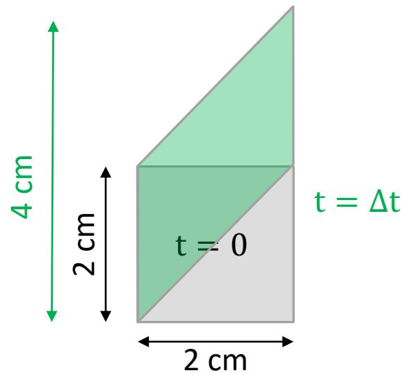
Find out the deformation gradient for the given deformation illustrated in the left figure.
