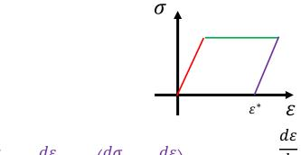
$$\frac{d\sigma}{dt} \neq 0, \frac{d\varepsilon}{dt} \neq 0, \left(\frac{d\sigma}{dt} = E\frac{d\varepsilon}{dt}\right)\sigma < Y \qquad \frac{d\varepsilon}{dt} = \frac{1}{E}\frac{d\sigma}{dt}, \sigma = E\varepsilon, \sigma < Y$$
