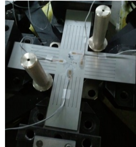
Digital image correlation by tracking displacement field u(X, Y)
