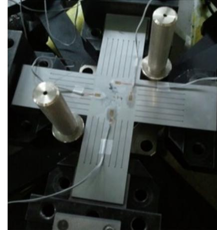
Strain field measurement (2D area)
