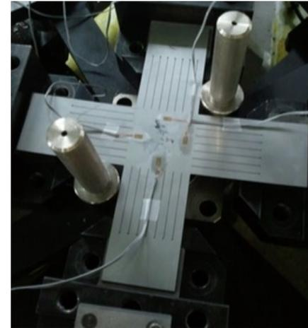
Strain field measurement (2D area)
