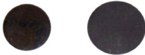
Fig. 4.4 Disk compression specimens for TWIP940 before (left) and after (right) deformation. The left one is original, the right one is deformed.
